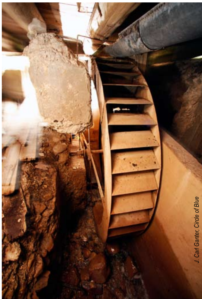
Louis DeYoung installed this waterwheel along a diverted stream and used the power it generated to do everything from blacksmithing to powering some of the first residential light bulbs in the area.
